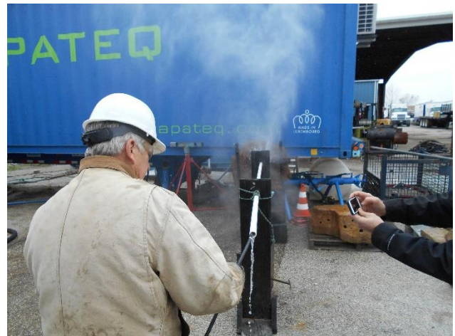
Figure 2 Sample holder and hose supporting tube
