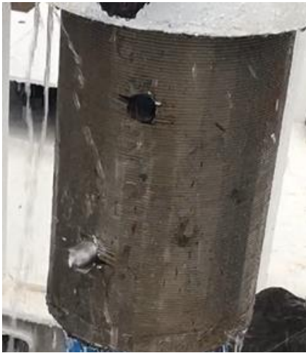
Figuur 11 Result milling through wirewrapp screen ECW
