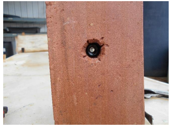
Figuur 5 results Trias sandstone with dynamic nozzle
