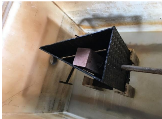
Figure 2 Sample holder and hose supporting tube
